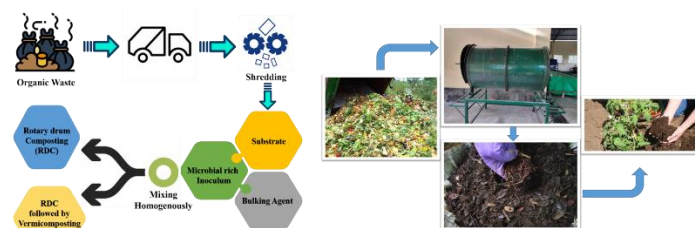
Fig. 1. The methodology adopted and the steps involving the composting process.
