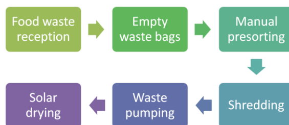
Fig. 1. Outline of the solar drying pilot plant process.
